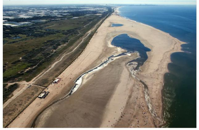
Every year, the sea takes sand from the Dutch coast. This loss of sand is replenished every five years by depositing sand on the beaches and in the offshore area to guarantee the high level of flood protection of the Netherlands. These replenishment operations do the job, but Dutch coastal scientists asked themselves: can we protect the coast in a more sustainable and natural way? They introduced a new concept of coastal protection: the Sand Motor (or Sand Engine).
